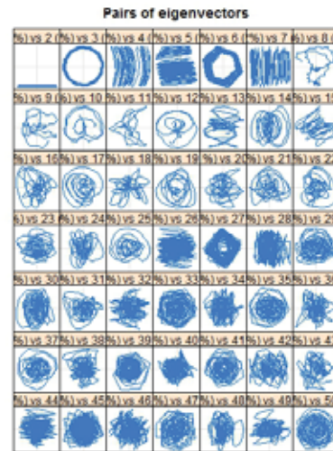
(b) Pairs of eigenvectors extracted with MSSA
